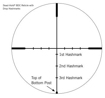
**NOTE:** This Vortex® riflescope uses a second focal plane reticle design and the listed BDC yardages will be valid at the highest magnification for most models. For 6–24x50 models, the listed BDC yardages will only be valid with the magnification set at 18x (indicated by a red mark on the magnification ring).
